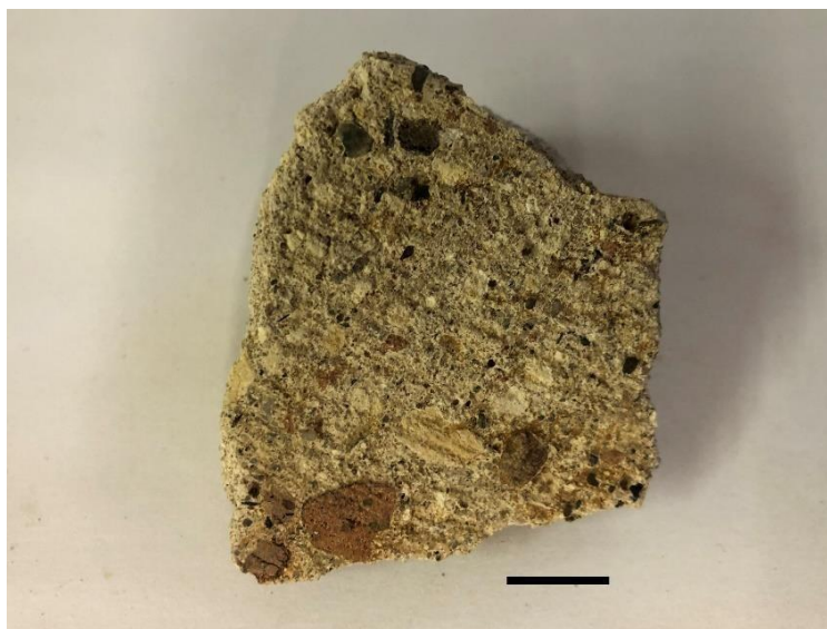
Figure 1. Image showing a freshly sawn face of the mortar. Scale bar = 10mm.
