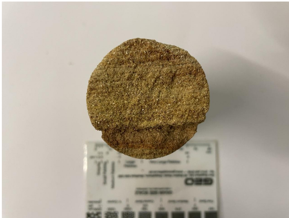
Plate 1. Image of the sample as received. Note the laminated texture and slight pink hue. Scale is in mm.
