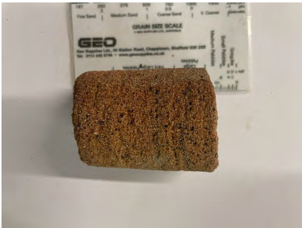
Plate 1. Image of the sample as received. Note the black speckling caused by Fe-oxides. Scale is in mm.
