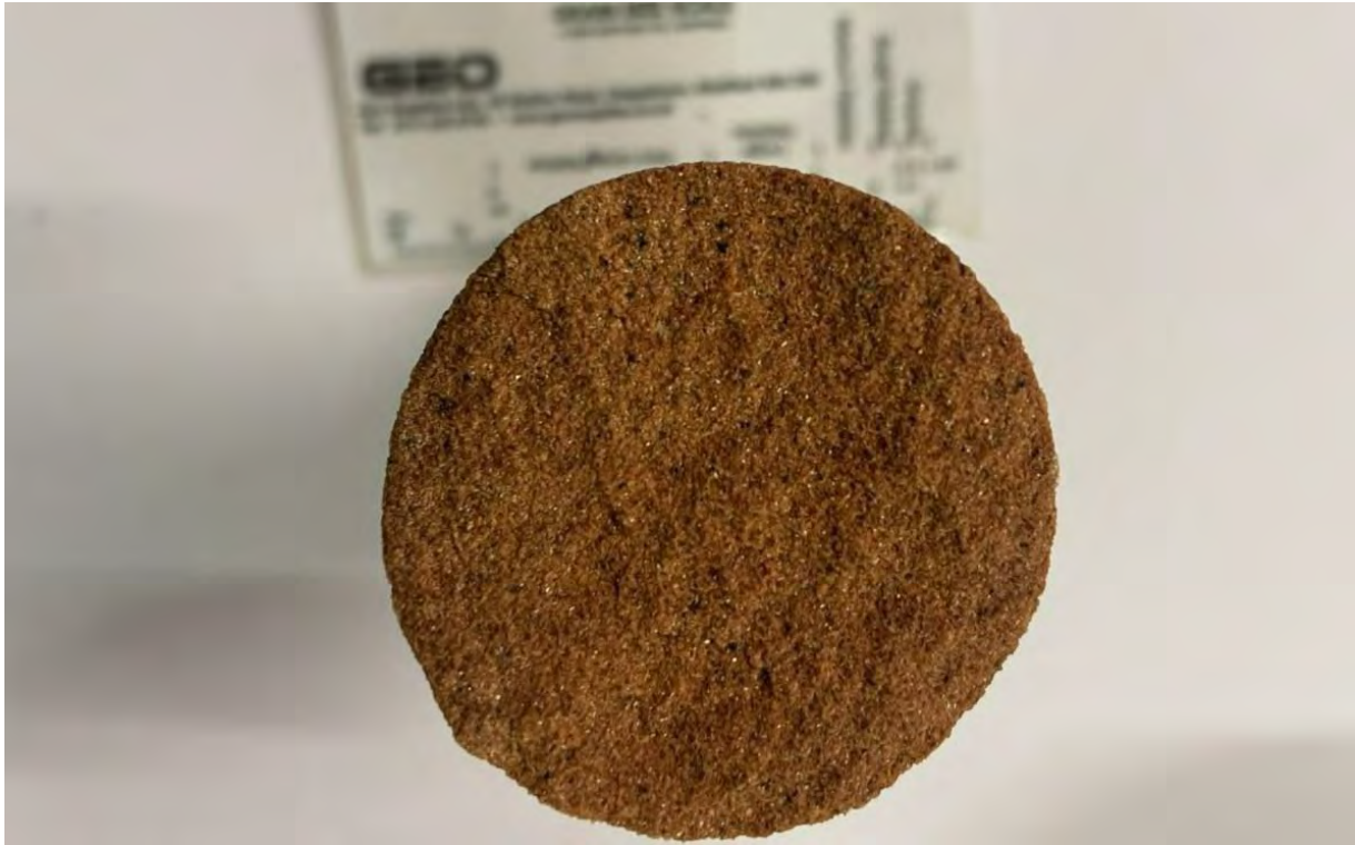
Plate 1. Image of the sample as received. Note the black speckling caused by Fe-oxides. Scale is in mm.
