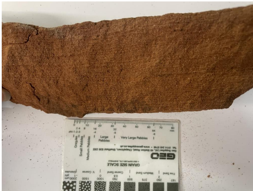
Plate 1. Image of the sample as received. Note the fine laminations in the stone. Scale is in mm.
