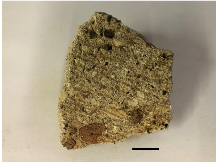
Figure 1. Image showing a freshly sawn face of the mortar. Scale bar = 10mm.
