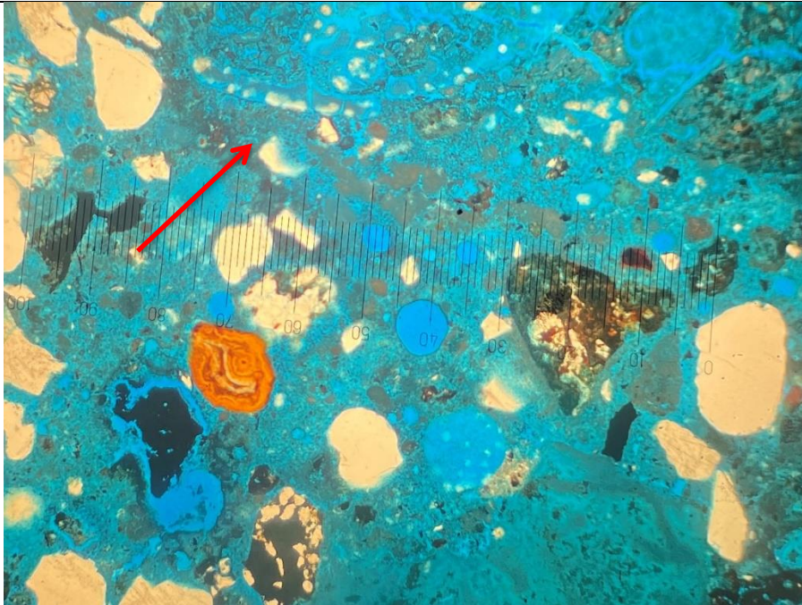
Figure 4. Thin section of the sample under plane polarised light. Pore spaces are highlighted in bright blue, while areas of dark/dull blue indicate the lime binder that has absorbed some of the blue dye. Most lime inclusions show a diffuse contact with the surrounding paste (highlighted by red arrow).
