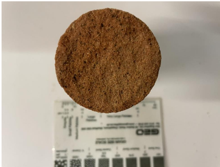
Plate 1. Image of the sample as received. Note the black speckling caused by Fe-oxides and carbonaceous matter. Scale is in mm.
