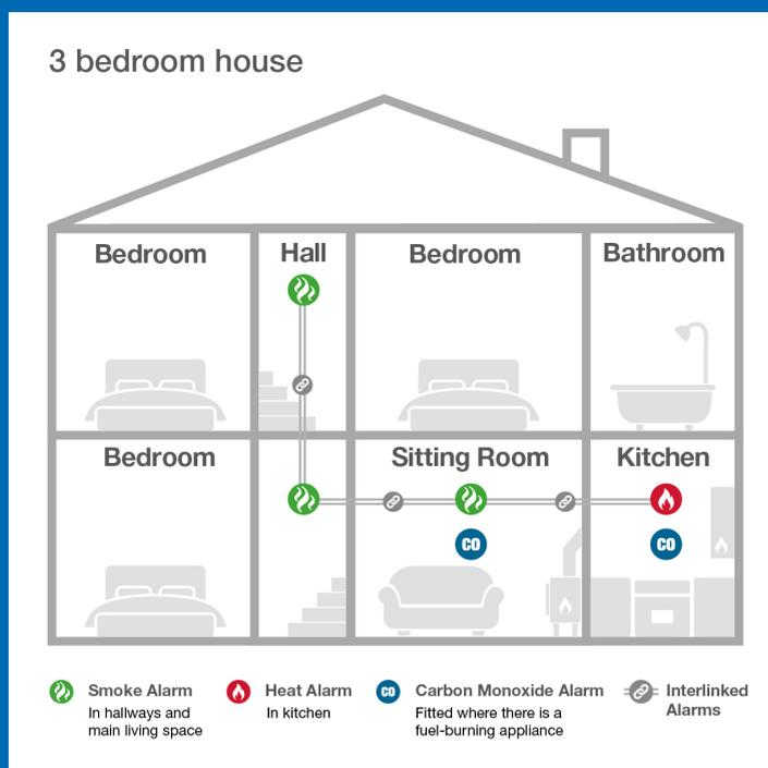
All alarms should be ceiling mounted and smoke and heat alarms interlinked.
